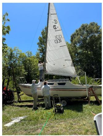
Whereas all the components of the boat were inspected, the principal project was to reinstall the mast step. That task was accomplished in comparatively short order. We were then able to step the mast and install a replacement boom from a Flying Scot. We weren't sure if the Scot boom would work but it was almost a perfect fit. With the boom in place, we were able to determine that several sails in the "Club's sail"
